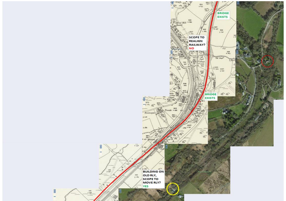
Section past former Lydford station, showing scope to realign railway to avoid house south of Lydford ↑
